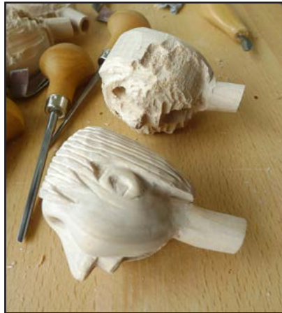
3. A head cut on a manual copy/carving machine.
