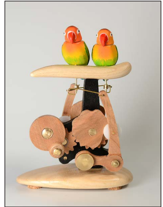
14. Lovebirds , using a multiple cam, open mechanism.
