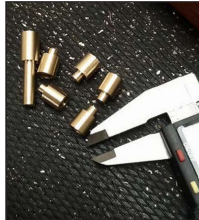
4. Turned-brass parts from the author's first lathe.
